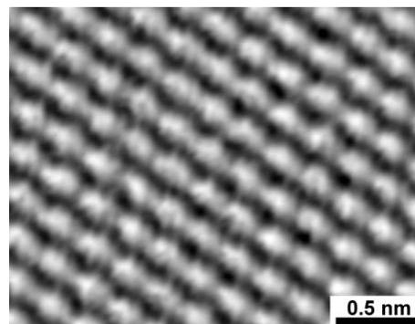
*STM image of graphite. Each big (“big”!) blob in this array is a ring of six smaller carbon atoms.*
