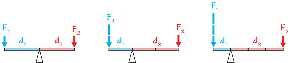
**Three class 1 levers in balance.** A class 1 lever has its fulcrum between effort and load. The effort and load could be at either end of these levers, depending on whether one wants to multiply or diminish the input force. (The first lever, with equal distances, neither multiplies nor diminishes force; it only changes the direction of the force.)
